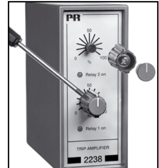
Picture 2: Removal of knobs.
